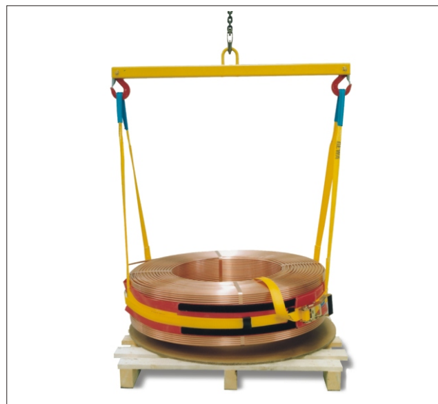
⑤ Lift coil with cross bar, vertically. (Coil should remain in a horizontal position. For safety reasons, do not transport above personnel.)
